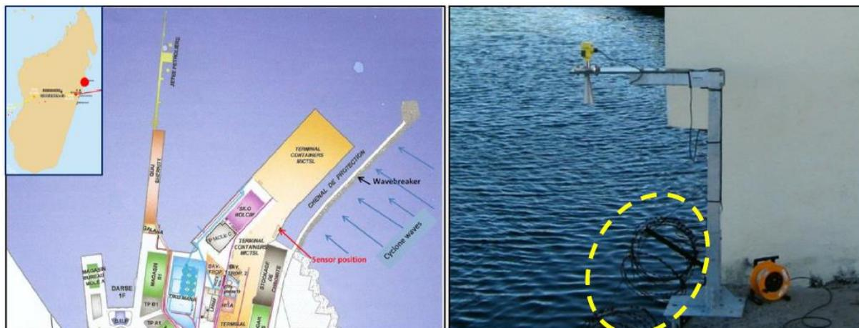
**Figure 75** - Vega Vegapuls62 radar sensor, Toamasina (Madagascar) tide gauge observatory (Source: SHOM [http://refmar.shom.fr/image/image\\_gallery?uuid=b4a9dc3f-de85-4b72-91e8-5ad1a864ca78&groupId=10227&t=1312547547320](http://refmar.shom.fr/image/image_gallery?uuid=b4a9dc3f-de85-4b72-91e8-5ad1a864ca78&groupId=10227&t=1312547547320)), as of 2012.
